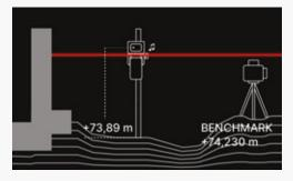
Move the computer head up on the rod until you read +73.890m on the display. When you receive a signal from the laser receiver, you know that you have the correct height +73.890m at the bottom of the rod.
